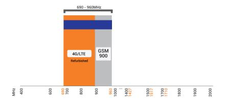
Indicates the LTE bands on which HELI-6 works
