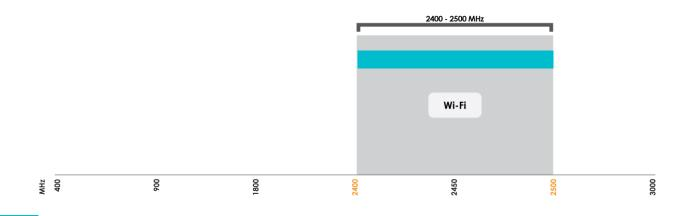
Indicates the WI-FI bands on which HELI-3-IS works
